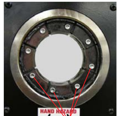
Grease Fitting Holes
